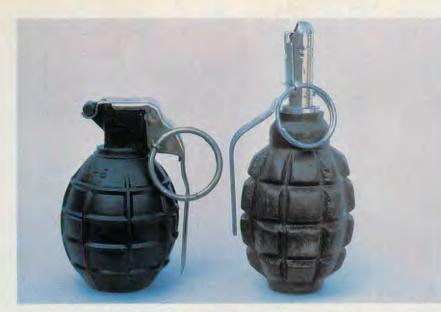
Side by side, USSR's M75 (left) and F1 represent one of the most advanced and one of the most primitive current-issue hand grenades.
